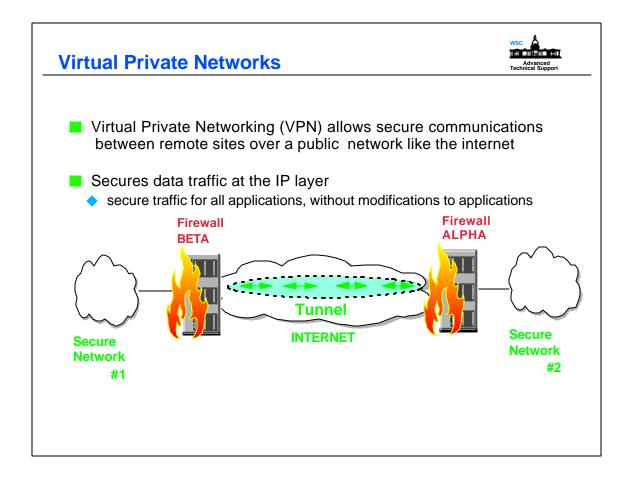
• Illustrated is a tunnel between two firewall hosts across the Internet. The two secure networks are in effect combined into a Virtual Private Network and it allows secure communications between the two hosts.
