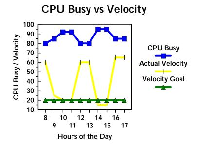
If a system is designed in this manner it may not be a good idea to allow discretionary work to be defined in the system. The production batch work's velocity will rise when there is more CPU and hence this work may now be eligible to be capped in favor of discretionary work if present. This may cause the overall throughput of the production batch work to suffer, as we allow discretionary batch to run.
