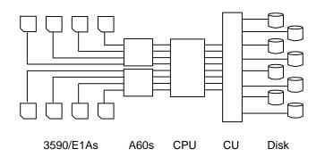
**Case #2.** Case#2 is restoring from 3590/A60s-E1As. Two A60s and eight E1As are used for the restore operation, providing two 1x4 strings. Throughput of 80.5 MBs/sec and an elapsed time of 1.3 hours. This throughput can only be achieved with ESS (Shark) or other disk
