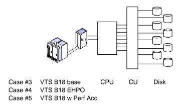
**Case #3, 4, & 5.** Cases #3, 4, & 5 are all restoring from a VTS. The three generations of currently available VTS are shown. Throughputs of 6, 18, and 40 MBs/sec are assumed for each of the three generations. These throughputs lead to elapsed restore times of 17.3, 5.8, and 2.3 hours respectively.
