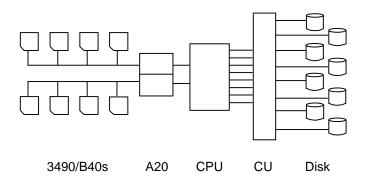
**Case #1.** Case #1 is restoring from 3490/A20-B40s. ESCON attached. One A20 and two B40s are used for the restore operation, providing two 1x4 strings. Throughput of 12.7 MBs/sec and an elapsed time of 8.2 hours. In case #1 the tape control unit is the constraint point.
