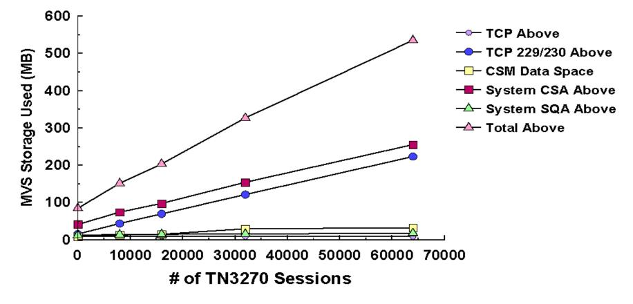
Storage usage (Above 16M line) of the TCP/IP Address Space and MVS System Storage (SQA and CSA) during TN3270 echoes (0 to 64000 users) when using z/OS V1R4 CS.
