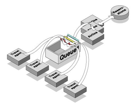
Figure 13. Load balancing. Large and fluctuating volumes of message traffic can be processed by multiple instances of a server program.
