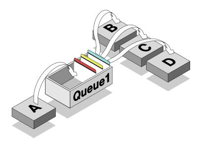
Figure 4. A one-to-many relationship between programs. In this example, program A distributes work among programs B, C, and D. Message flow could be two-way if necessary, with any of programs B, C, and D sending messages to program A.
