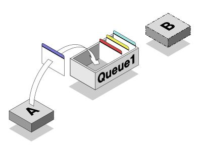
Figure 3. Either program can be busy or unavailable. In this example, program B is unavailable. The message intended for program B is retained in Queue 1 until the program is available again. (Message queues exist independently of the programs that use them, so both programs could be inactive at the same time; the message on its way from one program to the other is nonetheless retained in Queue 1 until program B is ready for it.)
