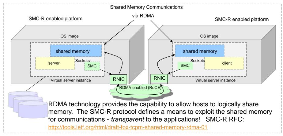
This solution is referred to as *SMC-R* (Shared Memory Communications over RDMA). SMC-R represents a sockets over RDMA protocol that provides a foundation for a complete solution meeting all of the described objectives. SMC-R is an RDMA model exploiting RDMA-writes (only) for all data movement.
