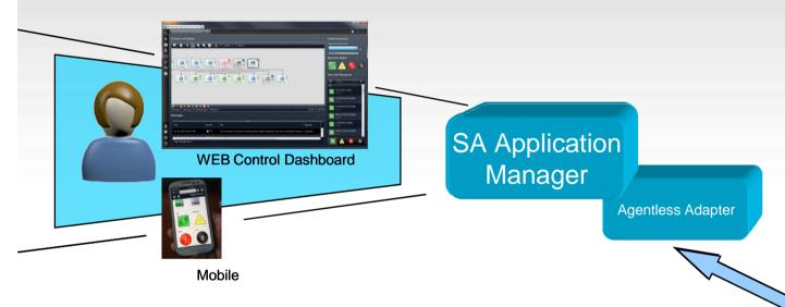
Agentless Adapter component of SA Application Manager controls availability state of any application running by using the standard "ssh" protocol
