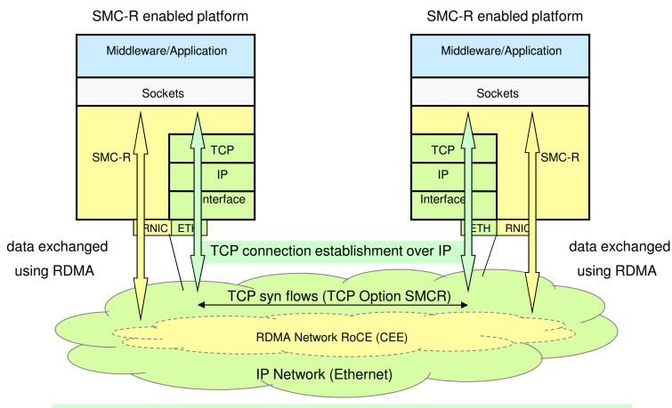
Dynamic (in-line) negotiation for SMC-R is initiated by presence of TCP Option (SMCR)
