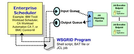
Integration with enterprise schedulers enables WebSphere batch to be introduced without disruption into existing processes
