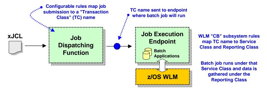
Classifying to a Service Class allows WAS z/OS to place work into separate servant regions based on Service Class Classifying to a Reporting Class allows WLM to gather system information for all work running under that Class
