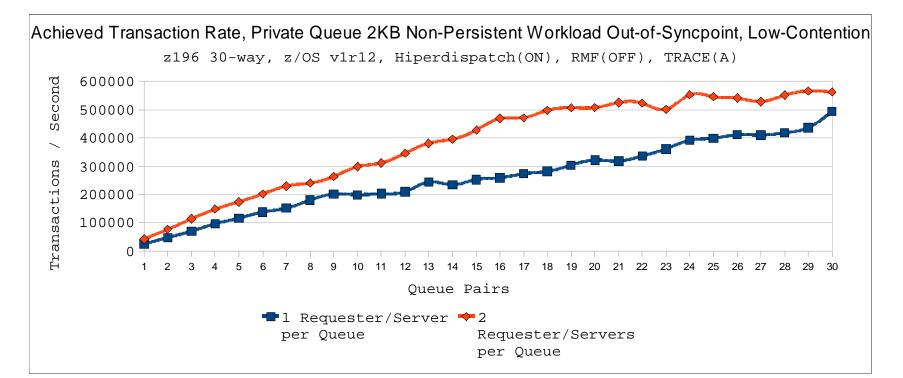
This measurement shows that MQ is able to exceed 550,000 transactions per second on a single queue manager running on a 30-processor LPAR
