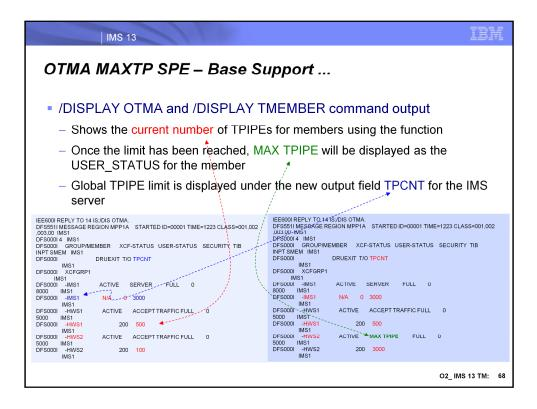
The /DISPLAY OTMA and /DISPLAY TMEMBER commands have been enhanced to allow the display output to show the current number of TPIPES for those OTMA members that have enabled the MAXTP support. Additionally, the 'MAX TPIPE' status is displayed when the limit has been reached.
