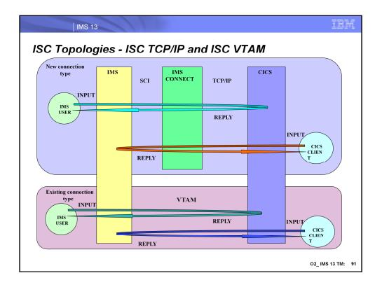
This visual depicts an IMS and CICS system supporting both VTAM and TCP/IP connection. For ISC TCP/IP, IMS communicates with IMS Connect via the Structured Call Interface (SCI). IMS Connect communicates with CICS via TCP/IP network.
