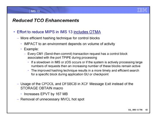
IMS 13 introduces a more efficient hashing mechanism for OTMA control blocks associated with transaction messages. The impact to a specific IMS environment depends on its use of OTMA.
