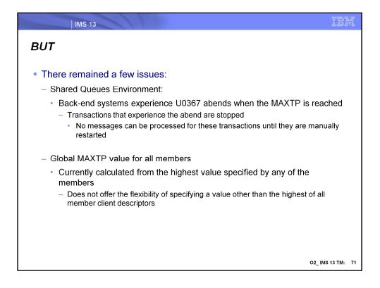
After application of the enhancements previously discussed there still remained a few issues. In a Shared Queues environment, U0367 abends occurred in back-end systems when the MAXTP condition was reached. Transactions that receive the abend are stopped and must be manually restarted.
