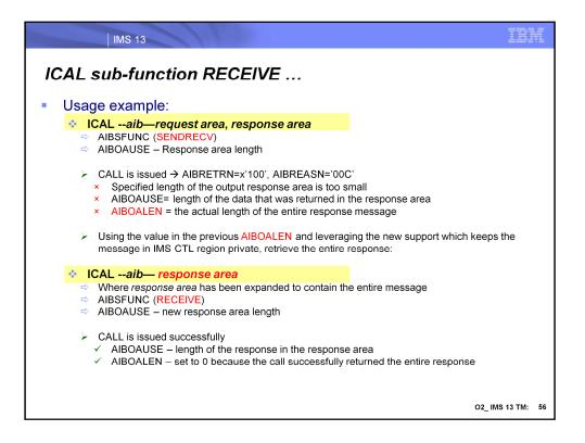
If an ICAL call with sub-function code SENDRECV is issued with an insufficient response buffer defined, the ICAL will be returned with AIB return code X'100' and AIB reason code X'00C'. A subsequent ICAL call with sub-function code RECEIVE can still be issued to retrieve the entire response message as long as it is defined with the expanded response buffer.
