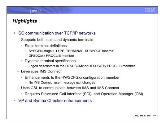
At a high level, the ISC support using TCP/IP protocols can be defined in IMS environments both statically and dynamically (ETO). It uses the SCI (structure call interface) of the CSL (common service layer) between IMS and IMS Connect in order to leverage the existing IMS Connect TCP/IP support.
