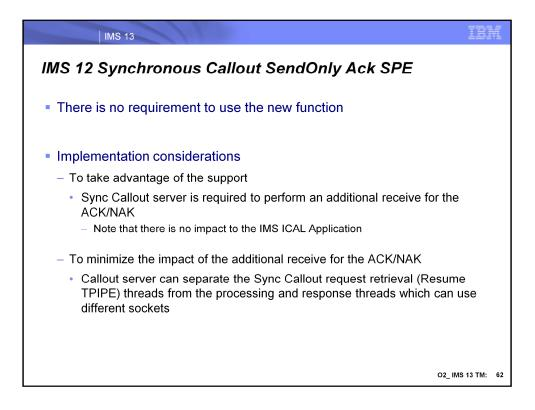
For a synchronous callout server application to take advantage of this new function, an additional receive for the ACK (acknowledgement) or NAK (negative acknowledgement or rejection) must be coded. This implementation does not impact or require any changes to the IMS application that issues the ICAL. The ACK/NAK is sent by OTMA.
