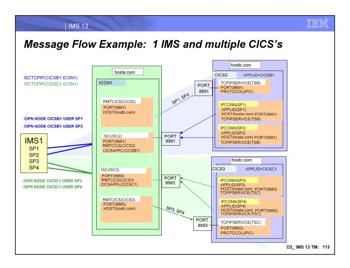
One IMS system can communicate with multiple CICS's using one IMS Connect.
