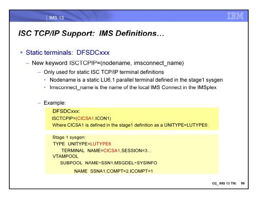
IMS enhances the DFSDCxxx PROCLIB member to provide static ISC TCP/IP terminal support for parallel sessions. Static ISC TCP/IP terminals do not support single ISC sessions. Because ISC terminals use VTAM support by default, the ISCTCPIP parameter in the DFSDCxxx PROCLIB member must be defined to enable TCP/IP for static LU 6.1 ISC terminals.
