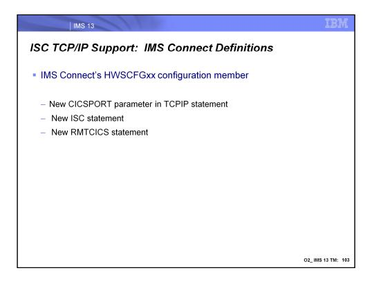
TCP/IP support for ISC is provided by IMS Connect and is defined by coding the appropriate configuration statements in the IMS Connect PROCLIB member. These include a new CICSPORT parameter in the existing TCPIP configuration statement, and new ISC as well as RMTCICS statements.
