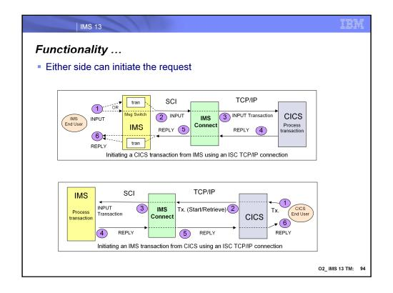
Initiating a CICS transaction from IMS using an ISC TCP/IP connection:
