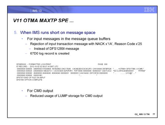
When IMS runs short on message queue space, input transactions are rejected with a NACK x'1A' reason x'25' instead of issuing a DFS1289I message. Additionally, a 67D0 log record will be produced.
