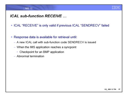
In order to issue an ICAL call with the sub-function code RECEIVE to retrieve the entire response message, the ICAL call with sub-function code SENDRECV must have previously been issued and returned with AIB return code X'100' and AIB reason code X'00C'.
