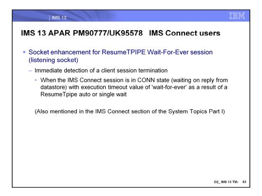
With this service the IMS Connect session that is in CONN state (waiting on reply from datastore) with execution timeout value of 'wait-for-ever' as a result of a ResumeTpipe 'auto' or 'single wait' will immediately detect a session termination of the client application.
