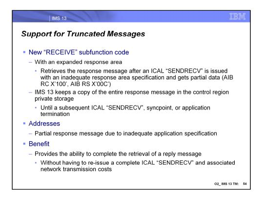
IMS 13 introduces a new subfunction of "RECEIVE" for the ICAL. This enhancement supports the retrieval of an entire response message if the original ICAL received partial data and an AIB return code of x'100' and reason code of x'00C'. By taking advantage of the new subfunction and expanding the response area in the call, the IMS application is able to retrieve the copy of the message that is temporarily kept in the IMS control region's private storage.
