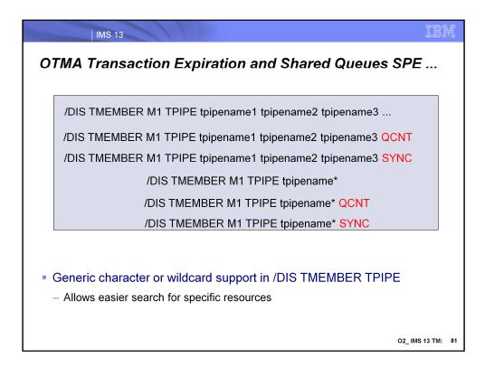
IMS improves OTMA usability by adding support for a generic character or wildcard at the end of the TPIPE name in the IMS command /DISPLAY TMEMBER TPIPE. By using the wildcard character, a series of TPIPE queues that are similarly named can be easily displayed. The generic form of the TPIPE name can also be used with the QCNT or SYNC keywords. Note that the TPIPE name with a generic character cannot be mixed with other TPIPE names.
