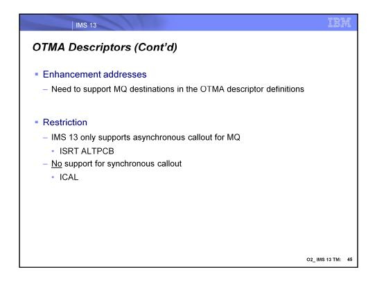
The new destination descriptor support for WebSphere MQ destinations cannot be used for synchronous callout ICAL calls.
