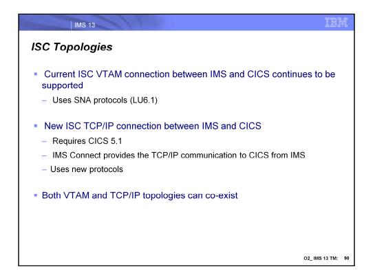
ISC VTAM (SNA LU 6.1) connections continue to be supported in IMS 13 alongside the new ISC TCP/IP capability. Connectivity to CICS using TCP/IP requires CICS 5.1. Both VTAM and TCP/IP connections can co-exist in both environments.
