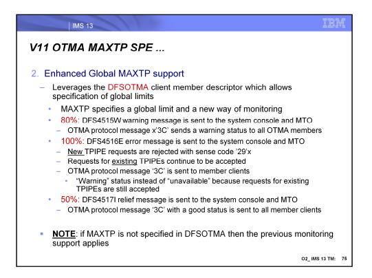
The enhancement for global MAXTP support leverages the DFSOTMA client descriptor and provides a MAXTP global limit for all the members. Once this is specified, IMS <u>no</u> longer uses the highest limit defined by any of the members. The MAXTP limit in DFSOTMA activates a new way of monitoring the TPIPE for all the members:
