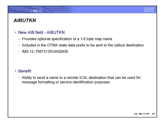
The DL/I ICAL call for synchronous callout can optionally use the first 8 bytes of a new AIBUTKN parameter to specify a map name in the application interface block (AIB). This value is passed in the OTMA state data prefix is can be uses by the remote destination of message formatting or service identification purposes.
