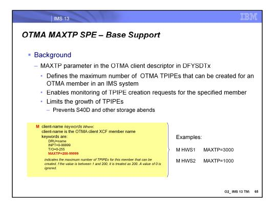
MAXTP is a parameter in the OTMA client descriptor that defines the maximum number of OTMA TPIPEs that can be created for that member. Once the parameter is defined, OTMA begins monitoring of the TPIPE creation requests. This capability is beneficial for limiting the unrestrained growth of TPIPES which could result in a S40D or other storage abend.
