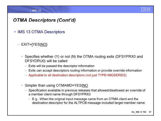
A new parameter EXIT= is added to the destination descriptor. When EXIT=YES is specified and OTMA routing exits (DFSYPRX0 and DFSYDRU0) are found in the IMS, the exits are allowed to override the routing information specified in the descriptor. Other IMS exits such as DFSYIOE0 are not affected by this new parameter. The default setting of EXIT is NO which means the OTMA routing exits, if found, cannot be called to override the routing information in the descriptor.
