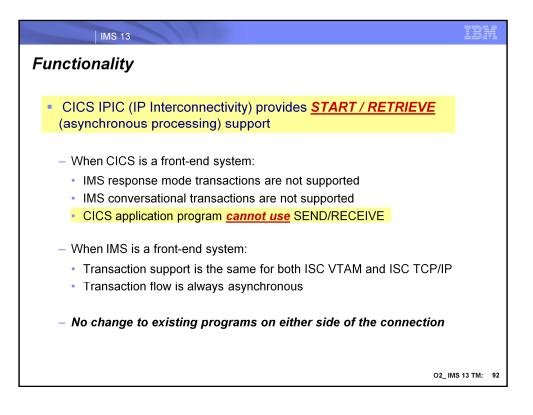
Connectivity between CICS and IMS only supports the START/RETRIEVE or asynchronous support in IMS 13. This means that when CICS is the front-end system, neither IMS response mode or conversational transactions can be invoked. Additionally, CICS application programs are not able to issue a SEND/RECEIVE (synchronous) type of request.
