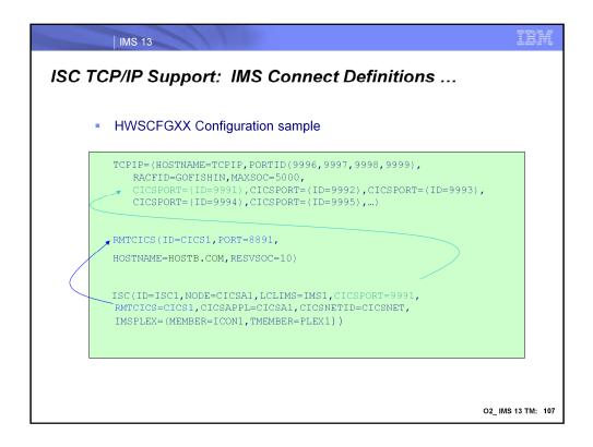
In this configuration example, note the RMTCICS definition. This shows that the local IMS Connect instance has been defined to use port 8891 for outbound communications with CICS. This is for establishing the SEND sockets from IMS Connect.
