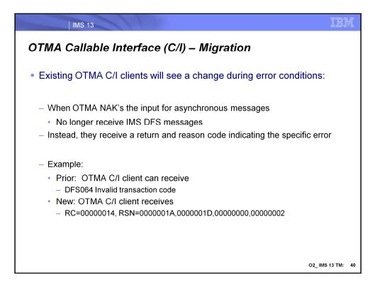
The OTMA C/I client using asynchronous messaging will no longer receive IMS DFS messages when the input is NAK'd by OTMA. OTMA C/I will be provided return and reason codes to indicate the specific error.
