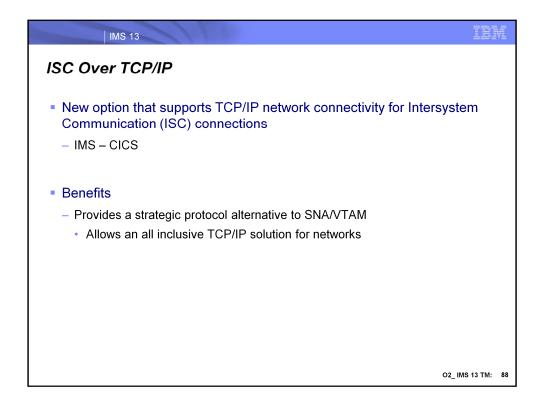
IMS 13 enhances Intersystem Communication (ISC) connectivity to included the TCP/IP protocol. This capability applies to connections between IMS and Customer Information Control System (CICS) systems. This new support provides a solution for environments that want to implement an all inclusive TCP/IP network environment.
