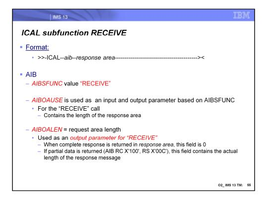
The format of the ICAL with a subfunction of "RECEIVE includes specification of the **aib** and a **response area** that can contain the entire message. Not all the *aib* fields are used for this call. The following apply:
