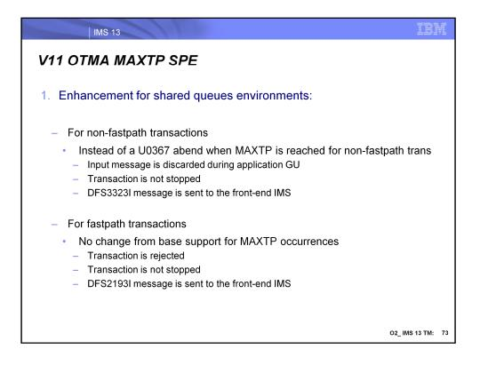
The first enhancement address the shared queues back-end system abends. After application of the SPE, when an IMS shared queues back-end system attempts to process a front-end initiated OTMA non-fastpath input transaction at application GU time and MAXTP is reached, abend U0367 does no longer occurs. Rather, the input message is discarded, the transaction is not stopped, and a DFS3323I message is sent to the front-end IMS to inform the OTMA client.
