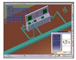
*Routing* links the various zones on a ship to a series of reservation envelopes that act as a "keep out" area for other services. This feature reduces conflicting uses of space while enforcing yard design standards.
