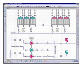
HVD supports the definition of HVAC diagrams, including general layout tools to place and locate
