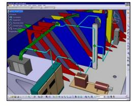
*3D Raceway and Conduit Design* is integrated with the *3D Cable Routing* application, which uses physical cable networks to manage cable routing definitions.
