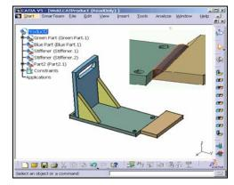
hidden-line-removal visualization mode of the assembly. 2D weld annotations are also created automatically. Within the 3D design, the mass and inertia of the weld ribbons are added to the mass and the inertia of the whole assembly so users who specify the weld material can perform relevant calculations.
