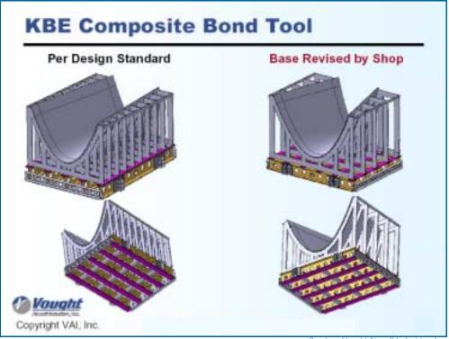
FIGURE 12 KBE Composite Bond Tool Standard vs. Revised
