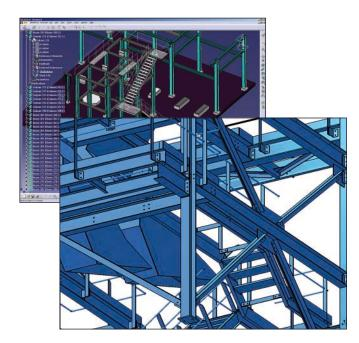
The PLM steel structure solution has been specifically designed to allow the overall structure to be divided into construction volumes, or zones, at any time prior to construction. This allows contractors to select the right zone at the optimal time, while enabling designers to achieve the best possible assembly breakdown structure.
