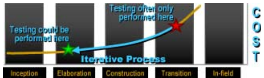
Figure 1: Problems Found Late in the Development Lifecycle Are Much More Costly to Fix.
