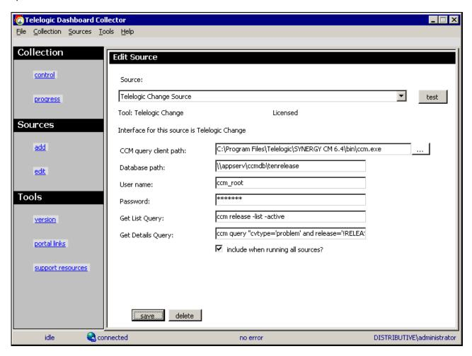
The "Path to client" is the location where Telelogic Change is installed on the local machine. The "Database path" is the location of the Telelogic Change Database. The Username and Password allows access to Change database.
