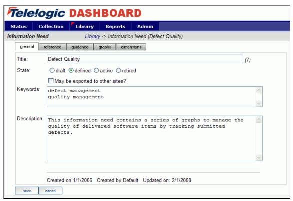
Selecting the **graphs** tab will list the graphs associated with the selected information need. In the sample below, Defect Quality has seven graphs defined. The various graph descriptions and series for each of the listed graphs can be edited here. When the Information Need is added to a unit, the graphs are applied to the data.
