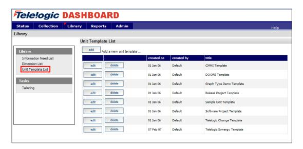
Select the **edit** button beside Telelogic Change Template. Selecting the **elements** subtab opens the page displaying the elements that have been assigned to the template.
