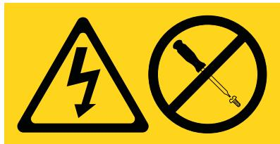
**DANGER:** Hazardous voltage, current, or energy levels are present inside any component that has this label attached. Do not open any cover or barrier that contains this label. (L001)
