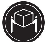
The weight of this part or unit is between 18 and 32 kg (39.7 and 70.5 lb). It takes two persons to safely lift this part or unit. (C009)
