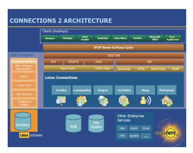
Figure 2. Lotus® Connections Architecture
