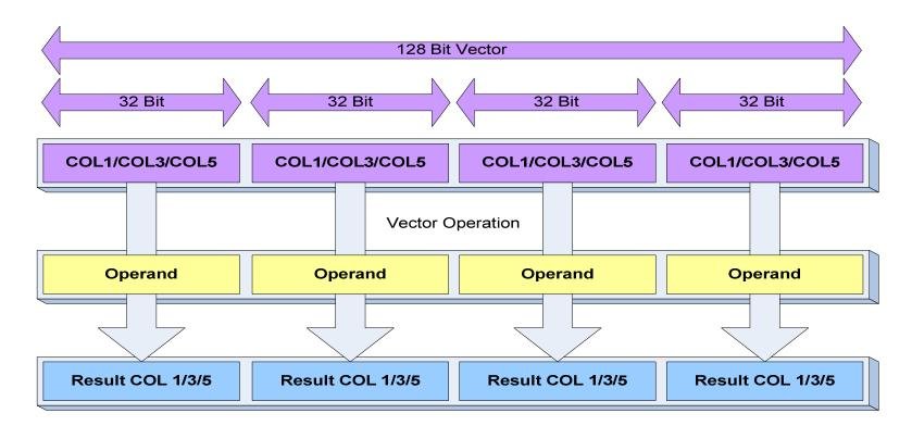
Packing multiple rows from the same bank into a 128-bit register permits **yet another level of parallelism – SIMD** (Single-Instruction, Multiple Data)!
