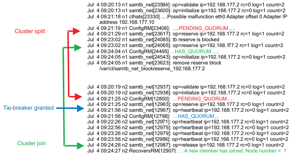
Figure 10. Two node cluster system logs
