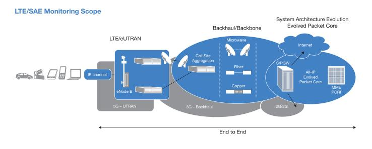
IBM Tivoli Netcool products manage the performance of the service provider communications network, including the LTE/ eUTRAN, the IP backhaul/backbone, SAE/EPC and end to end.
