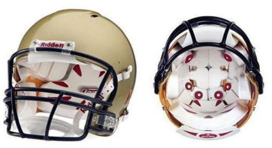
What looks like six marshmallows stuffed between the helmet's padding and the outside shell are actually foam-encased sensors that measure the acceleration of a player's head during a hit.
