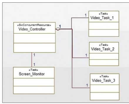
Figure 2: Concurrent task structure of a video player modeled in IBM Rational Rhapsody® software
