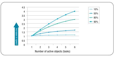
Figure 1: Applying Amdahl's law to predict the extent of speed gain as a function of parallel threads in a system
