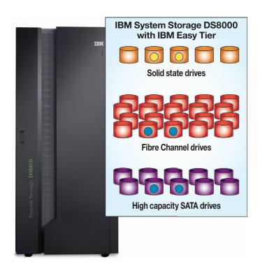
IBM Easy Tier® technology, shown here with the System Storage DS8000, automatically sends data to the most appropriate type of disk based on its frequency of use and importance, helping save money in disk purchases and enabling a more efficient use of storage resources.
