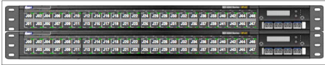
Figure 7-6 Two 1000BASE-T TOR switches
