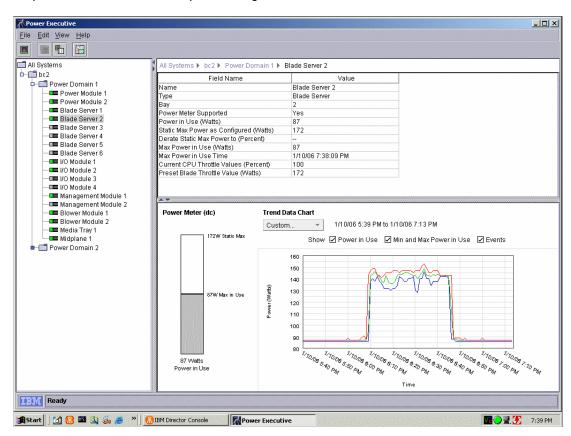
**Figure 1.** IBM PowerExecutive showing power measurement information for a single BladeCenter server
