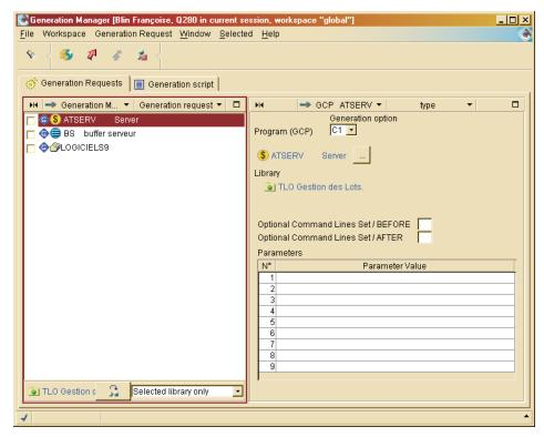
• The other tab is subdivided into two parts which initially display, if any, the user's command line set. These lines are created by an Administrator in the User browser.
