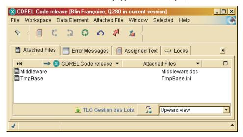
Once an External File instance is attached, cross-references are automatically created between the File and the instance which calls it.
