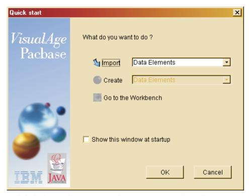
By default, the Quick Start smartguide pops up once you have chosen your connection context to AD workbench. To inhibit this option, uncheck the 'Show the window at startup' box; you will directly and systematically open the Workbench.
