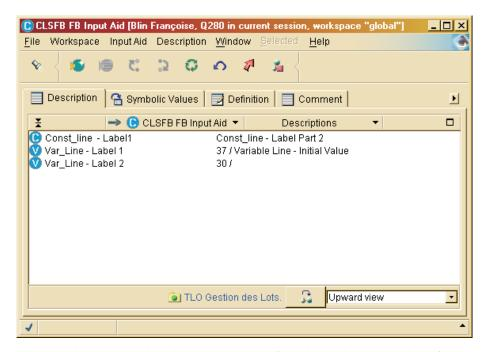
A Symbolic Values tab, where you may define the authorized values for editable parts, thus allowing input control on variable lines. This control is effective for variable lines whose editable part length is set to '3'. This constraint, due to internal reasons, has no impact on the actual length of authorized values.
