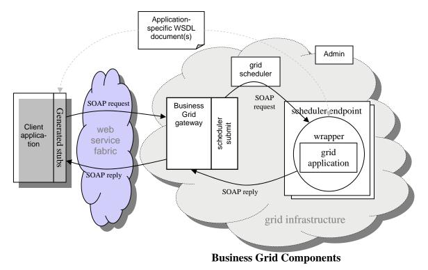
The following diagram shows a high-level component view of the Business Grid Components:
