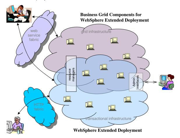
WebSphere Extended Deployment introduces the notion of dynamic application placement – that is, instances of a J2EE application can be started and stopped as warranted by current demand for the application and administratively-defined policy. Integrating WebSphere Extended Deployment with the Business Grid Components extends this concept to additionally include grid applications.
