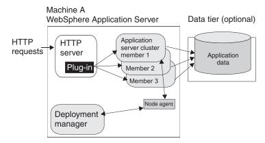
This topology illustrates a simple vertical scaling example, with multiple cluster members of an Application Server on machine A. You can also implement vertical scaling on more than one machine in a configuration. Combine vertical scaling with other topologies to boost performance and throughput.
