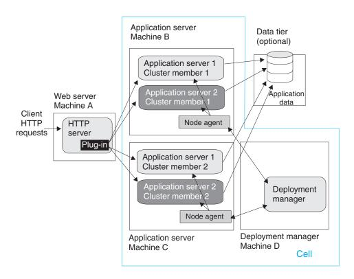
The example topology is a variation of the basic horizontal scaling topology. Cluster members are not hosted on just a single machine, but are distributed throughout all of the machines in the system. In this example, a cluster member is hosted on machines B and C. machine A serves as the Web server for the application and distributes client requests to the Application Server cluster members on each node.
