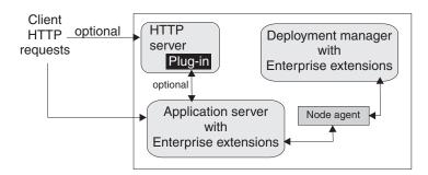
The Enterprise product installs a version of the base WebSphere Application Server product if the base product is not already on the machine. If it is on the machine, the Enterprise product checks to see if there are any required base features that are not already installed. If so, the Enterprise product installs the features.
