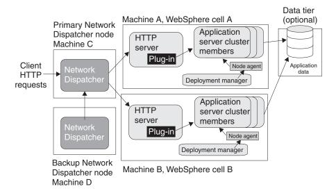
The example application runs simultaneously in two cells, each hosted on a different physical machine (machines A and B). Network Dispatcher is used to distribute incoming HTTP requests between the two cells, presenting a single image of the application to clients. A backup Network Dispatcher node provides failover support.
