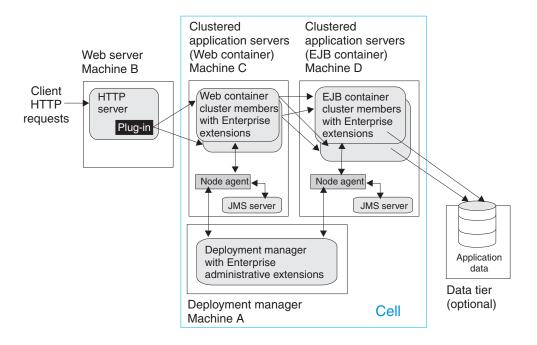
Installing the Enterprise product on machine A installs administrative extensions on the deployment manager node, adding options to the deployment manager administrative console for managing Application Server nodes that have Enterprise programming extensions. Installing the Enterprise product on machines C and D installs Enterprise programming extensions on the Application Server nodes. For example, machine D might have the Business Rules Beans feature of the Enterprise product, for example.
