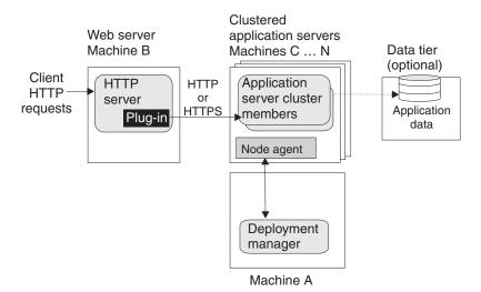
In the diagram, machine B hosts the Web server and receives HTTP requests from clients. The Web server forwards the requests to the Application Server on machine C, by using the HTTP or HTTPS protocol.
