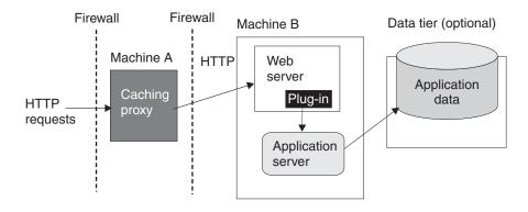
In this example, a reverse proxy resides in a demilitarized zone (DMZ) between the outer and inner firewalls. It listens on an HTTP port, typically port 80, for HTTP requests. The reverse proxy then forwards such requests to an HTTP server that resides on the same machine as WebSphere Application Server. After the requests are fulfilled, they are returned through the reverse proxy to the client, hiding the originating Web server.
