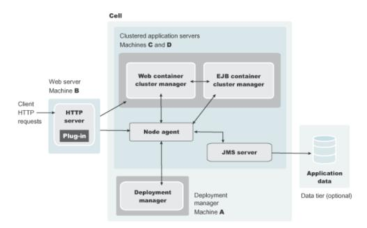
In this example, Web container cluster members (machine C) are closer (in a network sense) to the HTTP Server (machine B), which improves their response to client requests. Application Server processes that run enterprise beans (machine D) are closer in network terms to application data, which is represented in an application by entity beans and stored in a database on the data tier.
