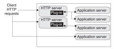
You can also install the base WebSphere Application Server product one time and use the **wsinstance** command to create multiple configuration instances. Configuration instances are fully functional Application Servers that share the run time and command binaries of the initial product installation. The following illustration shows an example of such a configuration.
