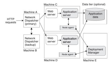
You normally configure a backup node for the Dispatcher machine, to eliminate it as a single point of failure. In this example, you can set up the backup Dispatcher node (machine B) to take over if the primary Dispatcher node (machine A) fails.
