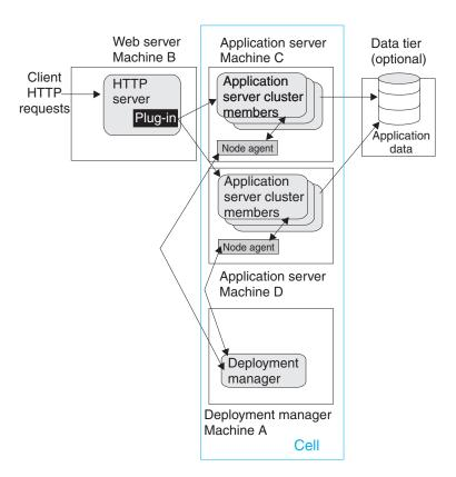
In this example, the Web server on machine B distributes requests to clustered Application Servers on machines C and D. Cluster members on machines C and D are created in the same cluster.
