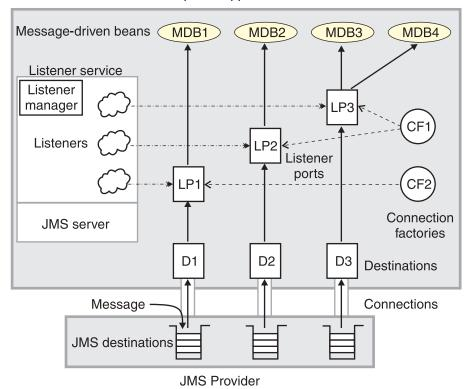
The *message listener service* is an extension to the JMS functions of the JMS provider and provides a *listener manager*, which controls and monitors one or more JMS *listeners*.
