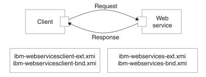
The client generates a request which is then handled by the client Web services engine. It reads the client security configuration and applies the security defined in
