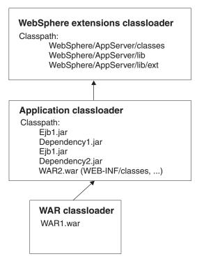
The following example shows that when the application class-loader policy of an application server is set to MULTIPLE, each application on the server has its own class loader. An application class loader also loads its Web modules if the application's WAR class-loader policy is set to APPLICATION. If the policy is set to MODULE, then a Web module uses its own class loader.
