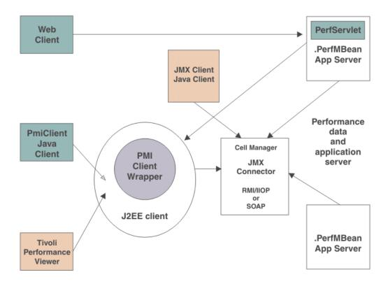
The figure shows the overall PMI architecture. On the right side, the server updates and keeps PMI data in memory. The left side displays a Web client, Java client and JMX client retrieving the performance data.
