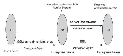
Scenario Explanation: This is an example of a pure Java client, C, accessing a secure enterprise bean on S1. C authenticates to S1 using SSL client certificates. S1 maps the cn of the DN in the certificate to a user in the local registry. The user in this case is "bob." The enterprise bean code on S1 accesses another enterprise bean on S2. Because the RunAs mode is system, the invocation credential is set as "server1" for any outbound requests.
