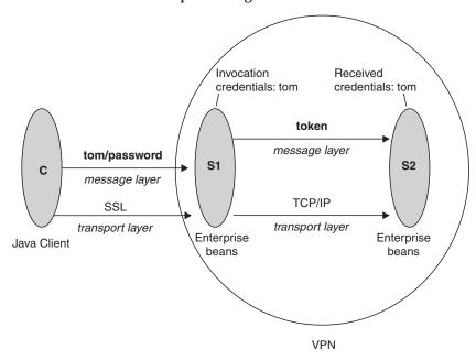
*Scenario Explanation:* This scenario illustrates the ability to choose TCP/IP as the transport when it is appropriate. In some cases, when two servers are on the same VPN, it may be appropriate to select TCP/IP as the transport for performance reasons since the VPN already encrypts the message.
