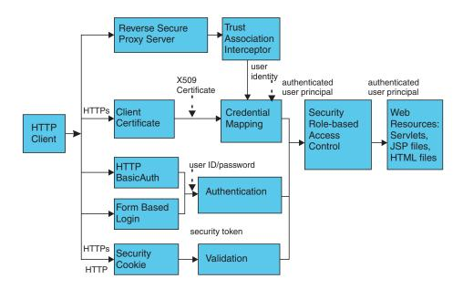
The Web security collaborator enforces role-based access control by using an access manager implementation. An access manager make authorization decision based on security policy derived from the deployment descriptor. An authenticated user principal is allowed to access the requested Servlet or JSP file if it has one of the
