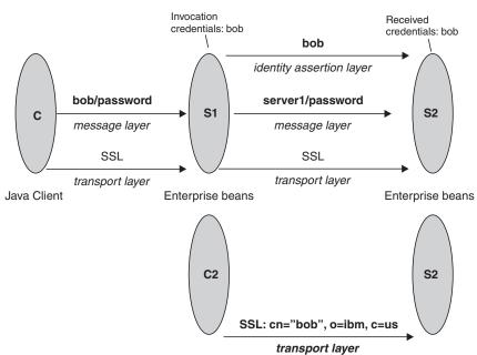
Scenario Explanation: This scenario is the same as Scenario 1 except for the interaction from client C2 to server S2. Therefore, the configuration of Scenario 1 still needs to be in place, but you have to modify server S2 slightly and add a configuration for client C2. There is no modification of the configuration for C1 or S1.
