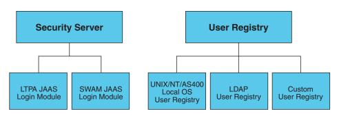
The product supports the J2EE Connector architecture and offers container managed authentication. It provides a default J2C principal/credential mapping module that basically maps any authenticated user credential to a PasswordCredential for the specified EIS security domain. The mapping module is a special JAAS LoginModule designed according to the Java 2 Connector and JAAS Specifications. Other mapping LoginModules can be plugged in.
