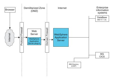
The WebSphere Application Server plug-in routes HTTP requests according to the virtual host and port configuration and URL pattern matching. Client authentication and finer grained access control are handled by WebSphere Application Server behind the firewall.
