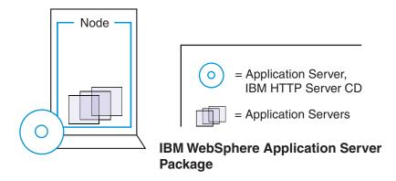
A Network Deployment installation can support a network of computer systems that are configured to run collaborating instances of a single server installation. Each computer having a single server installation is known as a node. The Network Deployment product provides centralized administration and workload management for a set of nodes, known as a (cell). A cell has a (master administrative repository) that stores all of the cell's configuration data.
