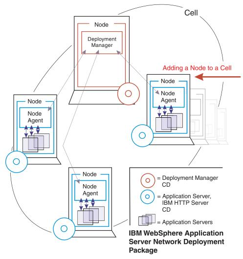
Administrative logic running in a node agent (keeps the configuration data of a node synchronized) with the configuration data of all nodes within a cell.
