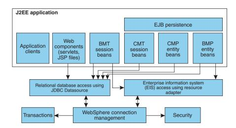
The J2EE Connector architecture defines a standard architecture that enables the integration of various enterprise information systems (EIS) with application servers and enterprise applications. It defines a standard resource adapter used by a Java application to connect to an EIS. This resource adapter can plug into the application server and, through the Common Client Interface (CCI), provide connectivity between the EIS, the application server, and the enterprise application.
