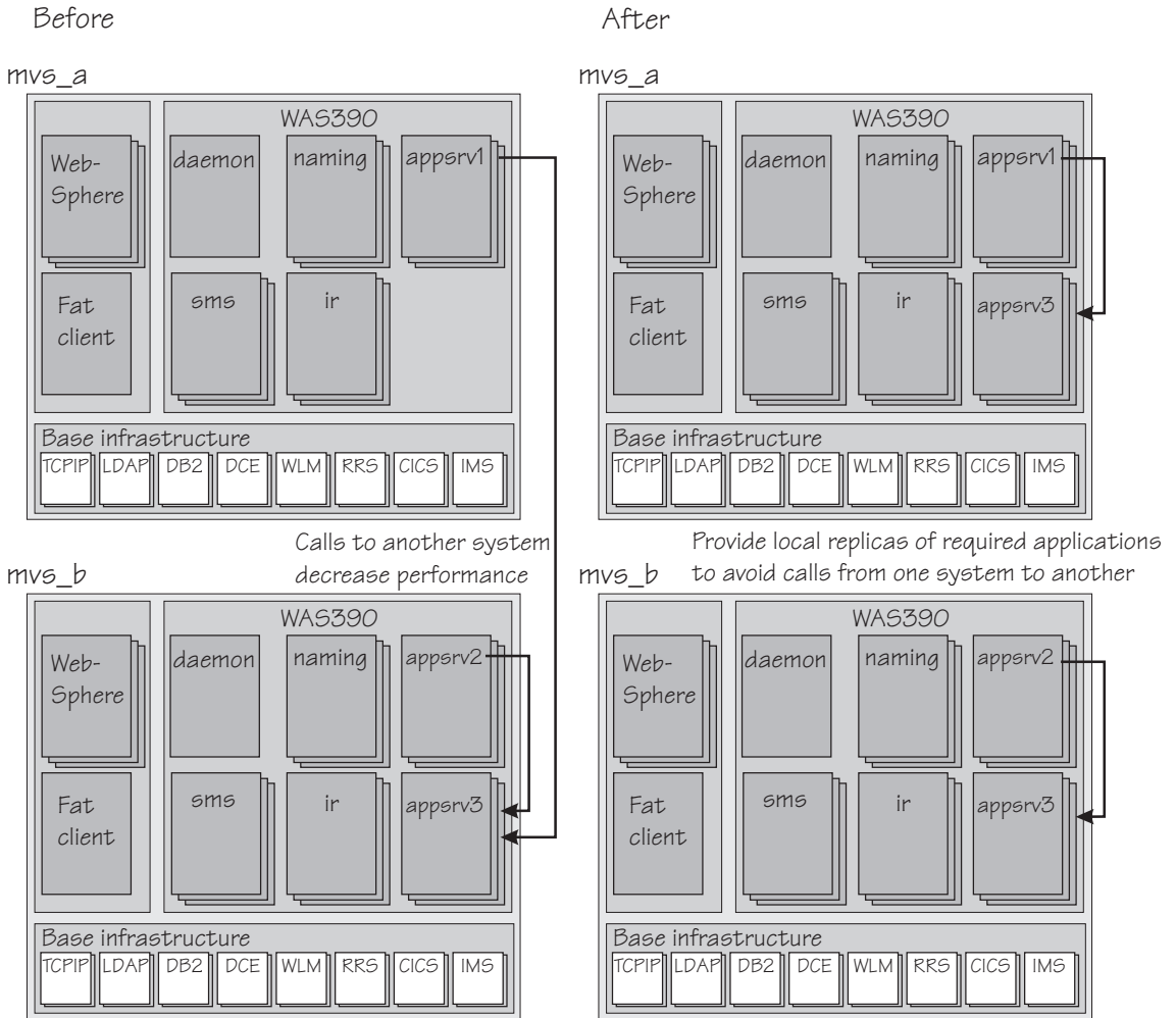
Figure 4. Having applications on a single system avoids calls from one system to another
