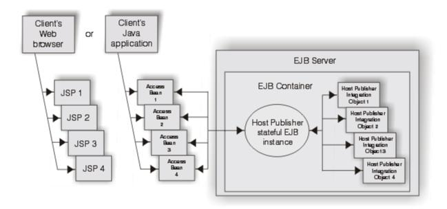
This above figure illustrates these concepts where the JSPs are executed in a Web container, the client Java application in a non-WebSphere JVM, and the Host Publisher EJB in a WebSphere EJB container.
