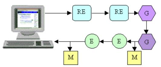
A WBI transaction. The HTTP data flows through a series of request editors (RE), generators (G), and response editors (E) before being returned to the client. Note that once one generator creates a response, other generators in the stream are ignored. Monitors (M) are also positioned at various points in the response stream.
