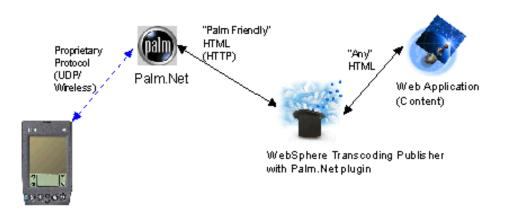
The Palm Device must be configured as described above. The proxy address is the address of the Palm.Net service, not of the WTP transcoding server.
