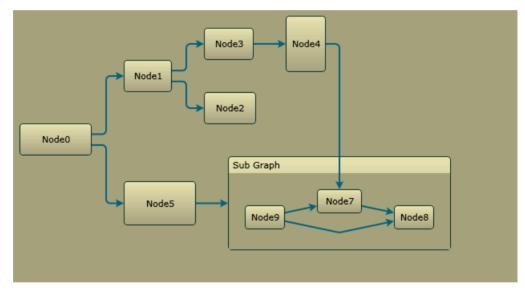
Note that the link between node 4 and node 7 is crossing graph boundaries. This is an integraph link (the start node is not in the same container than the link).
