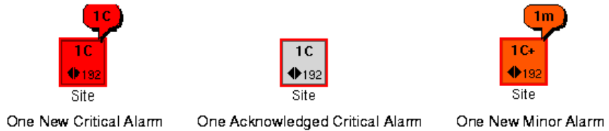
Network element with outstanding alarms
