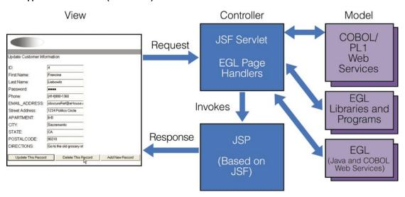
An EGL and JSF development environment can help support the development and integration of Web applications with COBOL and PL/I.
