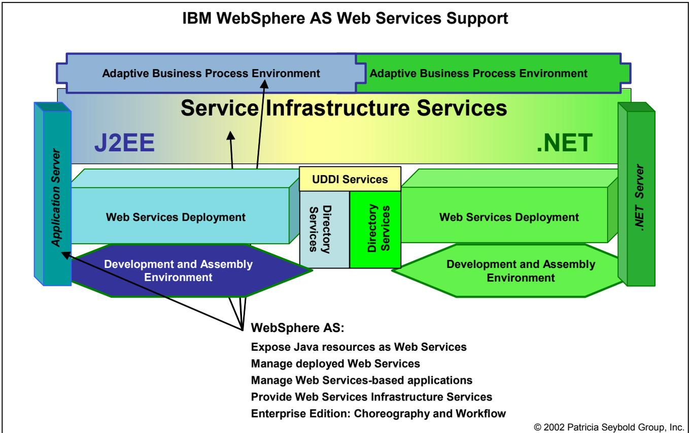
Illustration 2. WebSphere AS provides Web Services runtime, security, SOAP server, and client services; UDDI, WSDL, and XML support; and enables component deployment. WebSphere AS also provides Web Services Infrastructure Services and choreography support for Adaptive Business Process Environments.
