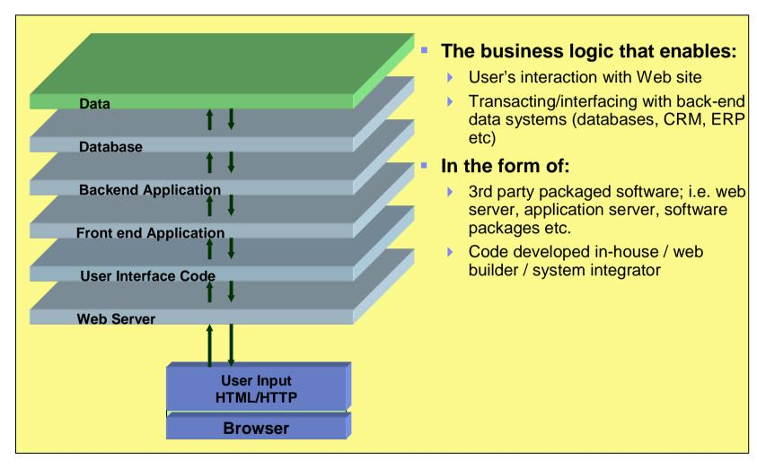
Input and Output flow through each layer of the application
