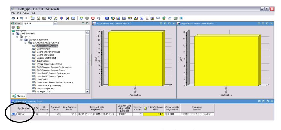
In this example, the application being monitoring is XCF (Cross Coupling Facility). The data set with the high response time is the Couple data set, which is a key resource in any environment.
