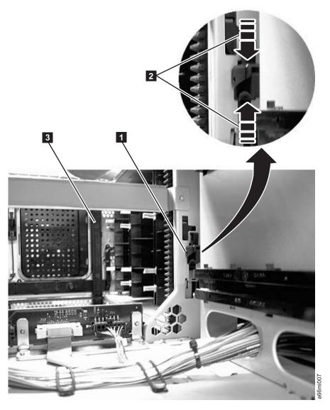
Figure 8-58. Removing a gear rack
