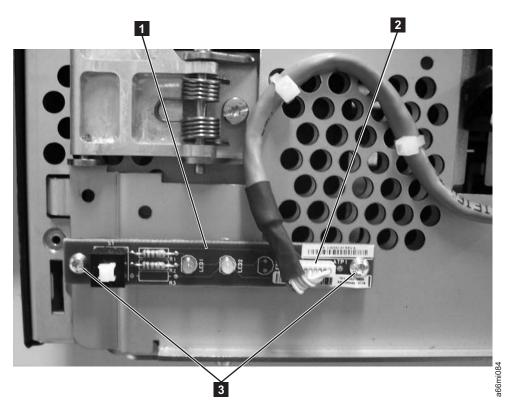
Figure 8-23. Power ON/OFF Button Assembly
