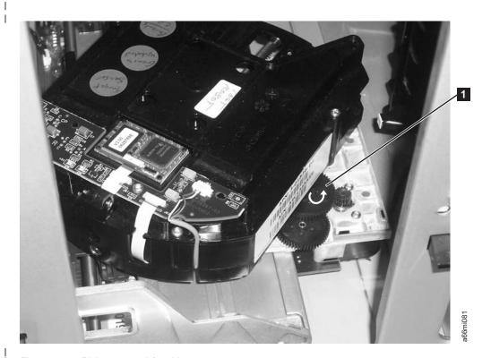
Figure 7-16. Picker rotated for drive gears access
