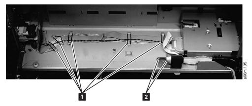
Figure 8-61. Cable assembly from the Operator Control Panel to the Backplane Connector Board
