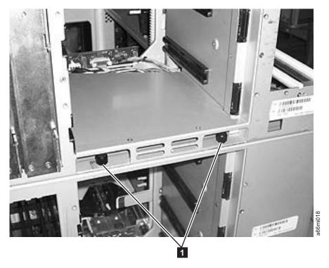
Figure 8-7. Control module rear thumb screws
