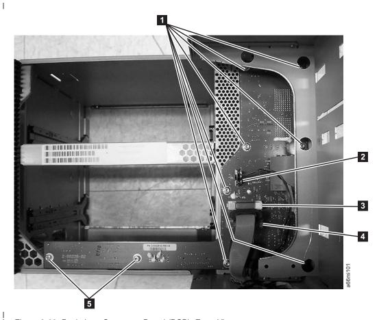
Figure 8-62. Backplane Connector Board (BCB), Front View
