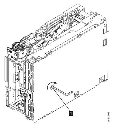
Figure 8-78. Using hex wrench to rewind tape into cartridge
