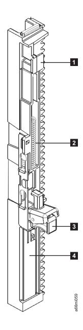
Figure 8-59. Gear rack (detail)
