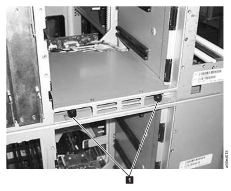
Figure 8-3. Control module rear thumb screws
