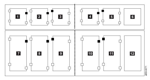
Figure 8-39. Correct fiducial placement
