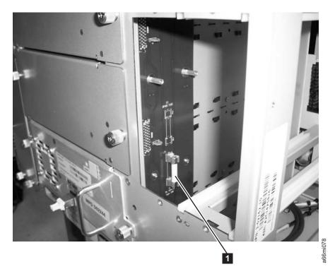
Figure 8-70. Drive power overload fuse
