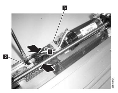
Figure 8-52. Y motor connector
