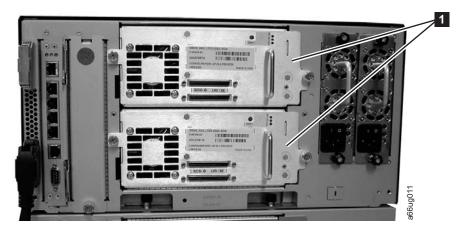
Figure 8-25. Control Module Drive Sled
