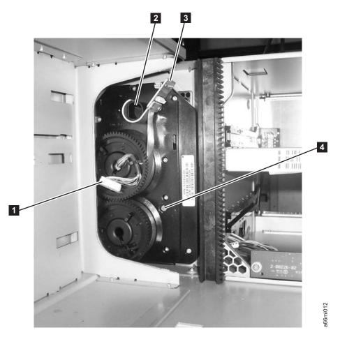
Figure 8-45. Securing Spooler flat cable
