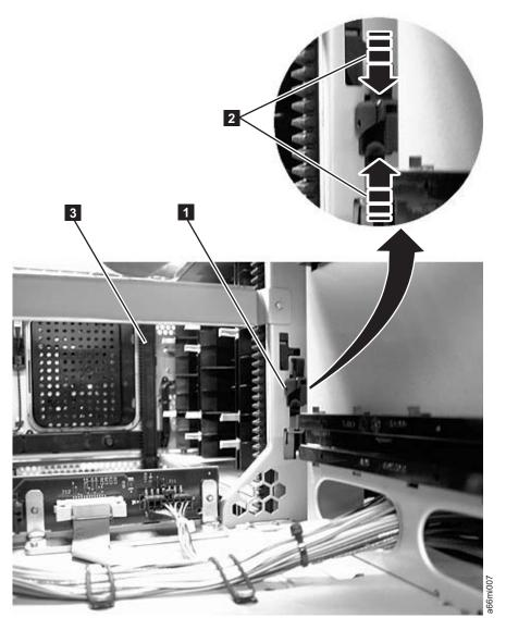
Figure 8-10. Gear rack
