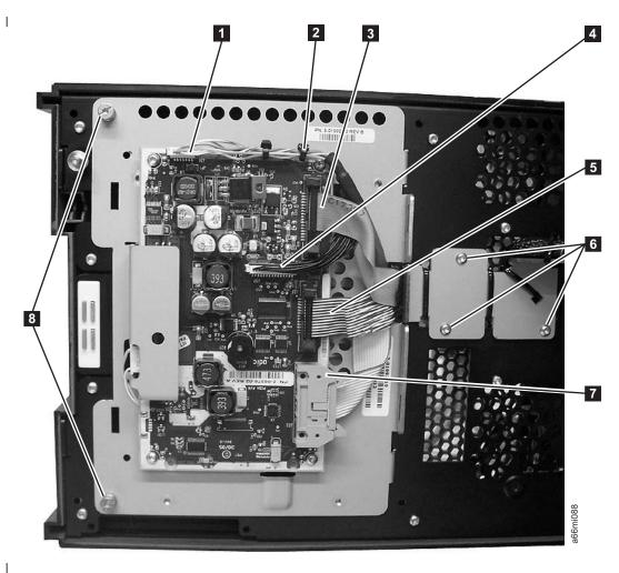
Figure 8-63. Operator Panel Cable Connectors
