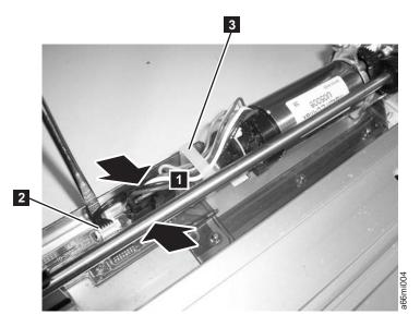
Figure 8-51. Y motor connector
