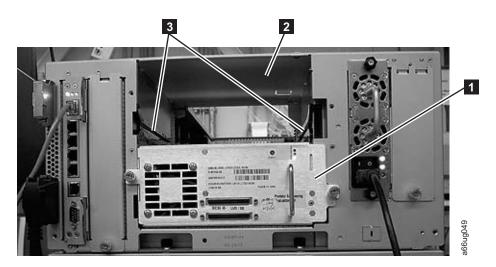
Figure 8-26. Drive sled slot
