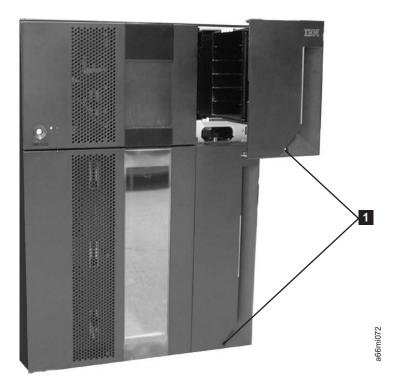
Figure 7-17. Access holes for manually unlocking I/O Station doors
