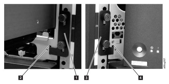
Figure 8-9. Removing the rack ears (Control Module shown)
