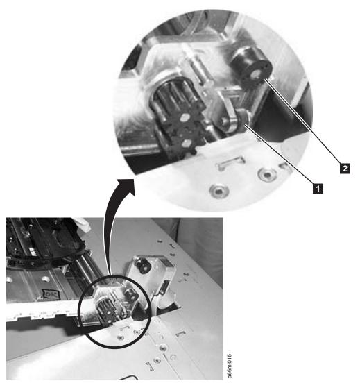
Figure 8-36. Guide rollers on Y-axis/Picker Assembly
