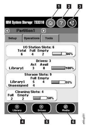
Figure 4-1. Operator Panel common header elements and subsystem status buttons
