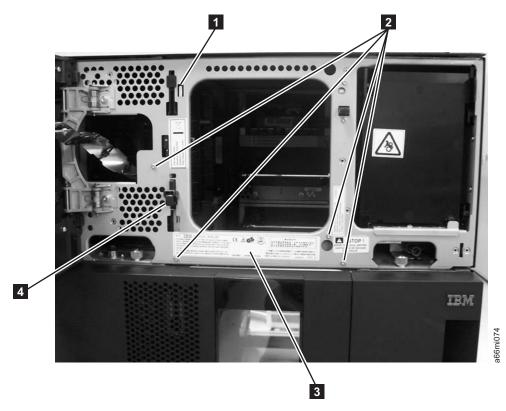
Figure 8-64. Four screws on front of door and plastic cable guide
