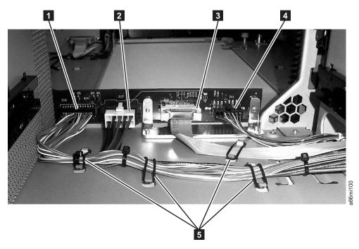
Figure 8-66. Backplane Connector Board (BCB), Rear View
