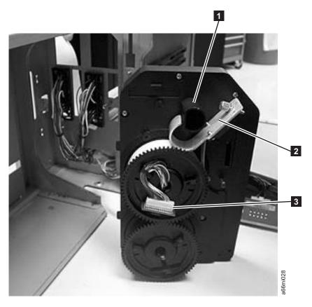
Figure 3-11. Cable spool assembly
