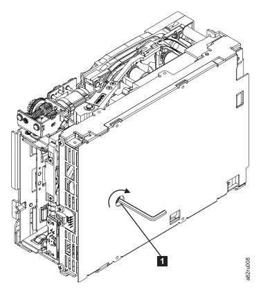
Figure 8-81. Using hex wrench to rewind tape into cartridge
