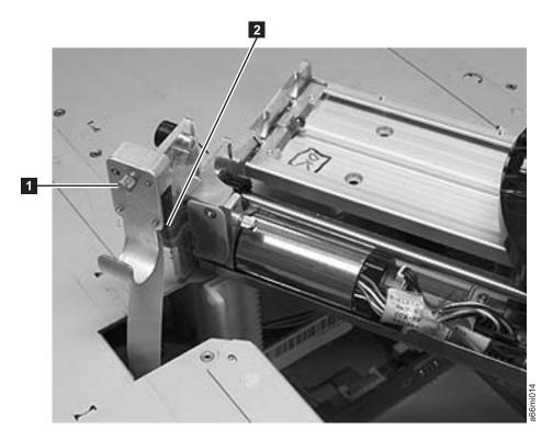
Figure 8-33. Thumb screw securing Cable Spool
