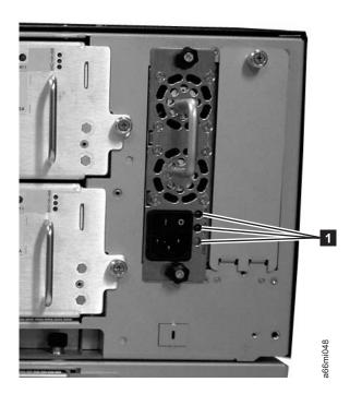
Figure 7-4. Power supply LEDs
