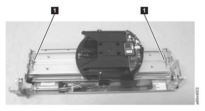
Figure 8-43. Thumb screws
