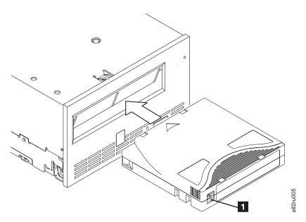
Figure D-2. Inserting a cartridge into the drive
