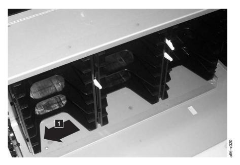
Figure 8-38. Removing a storage column
