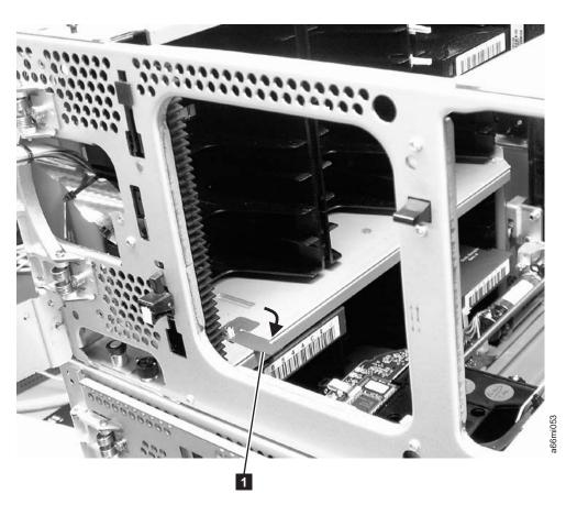
Figure 8-11. Picker assembly locking mechanism
