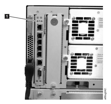
Figure 7-2. Library Control Blade LEDs
