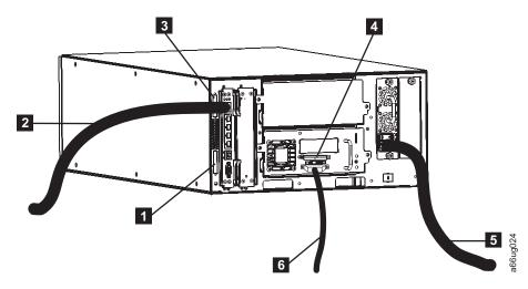
Figure 7-6. Cabling of a 5U Library with SCSI Drives
