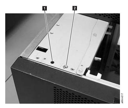
Figure 8-6. Alignment pin and front thumb screw receptacles
