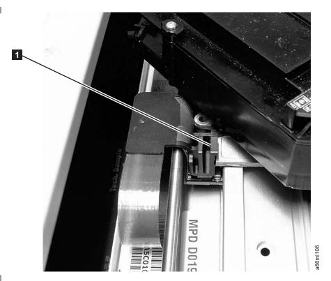
Figure 7-15. Picker assembly connector
