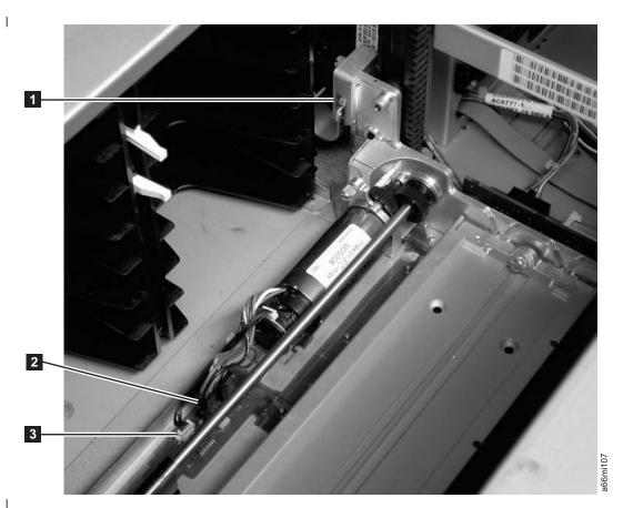
Figure 7-14. Y-axis and Y motor assembly connectors
