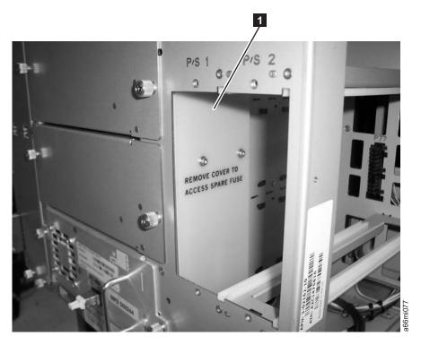
Figure 8-69. Drive power overload fuse cover plate
