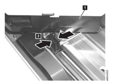
Figure 8-42. Flat cable connector
