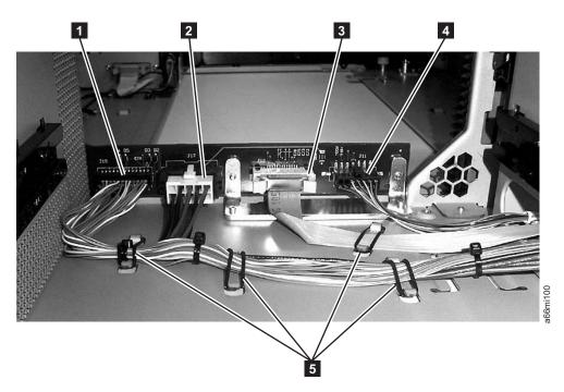
Figure 7-12. Backplane Connect Board connectors (back, drive sleds removed)
