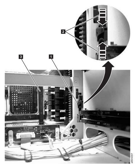
Figure 8-8. Gear racks and gear rack locking mechanism
