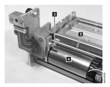
Figure 8-50. Correct Y motor position
