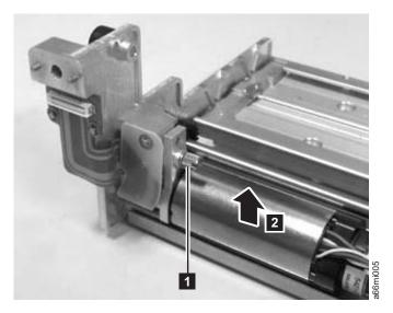
Figure 8-53. Y motor thumb screw
