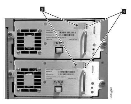
Figure 7-3. Tape drive LEDs
