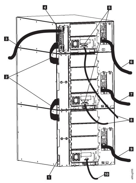
Figure 7-8. Cabling of a 23U Library with SCSI and Fibre Drives
