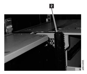
Figure 8-5. Gear racks (down and up)
