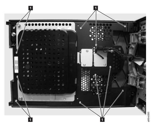
Figure 8-12. Control module Access Door screw locations
