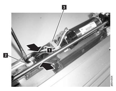
Figure 8-55. Y motor connector
