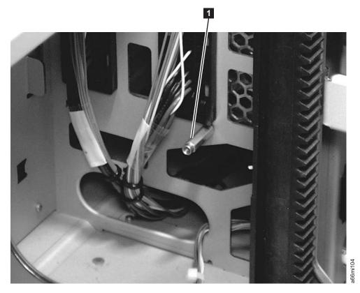
Figure 8-65. Hex stand-off behind the Cable Spool Assembly
