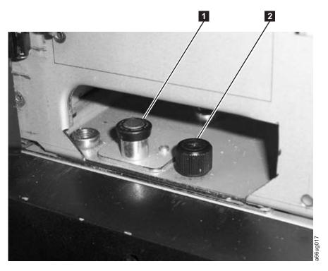
Figure 8-4. Alignment pin and front thumb screw
