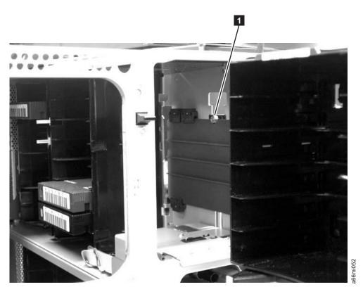
Figure 8-20. Silver roller locking the I/O Station slide in place
