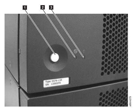
Figure 7-1. Power button LEDs
