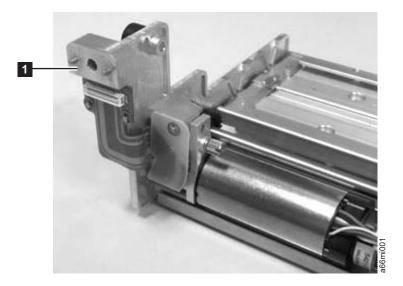
Figure 8-35. Thumbscrew securing Cable Spool
