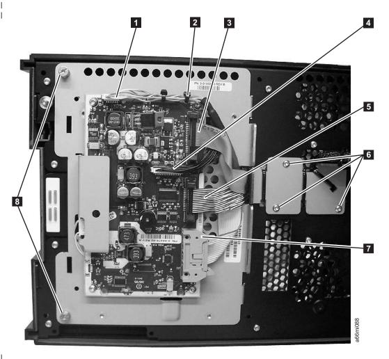
Figure 7-9. Operator panel connectors
