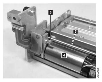
Figure 8-54. Correct Y motor position
