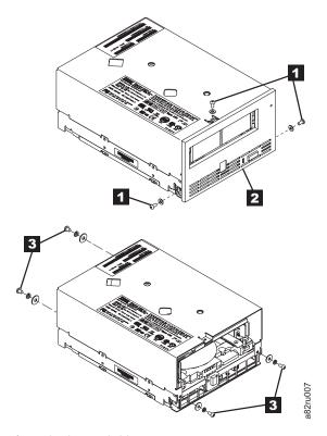
Figure 8-72. Removing the cover from the internal drive
