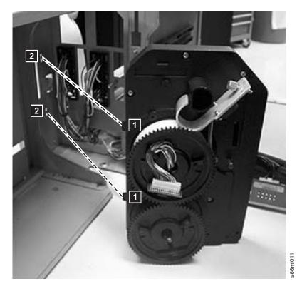
Figure 8-47. Cable Spool Assembly tabs
