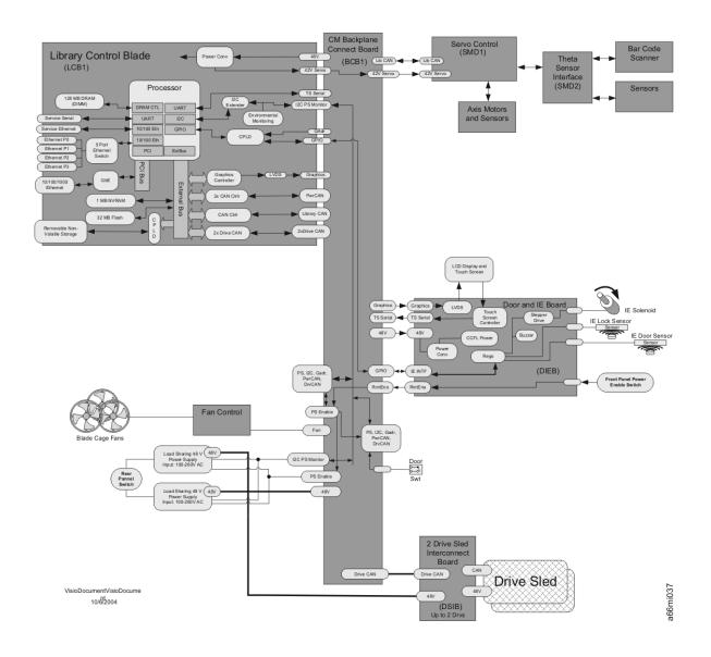
**Control Module and Expansion Module Electrical System**
