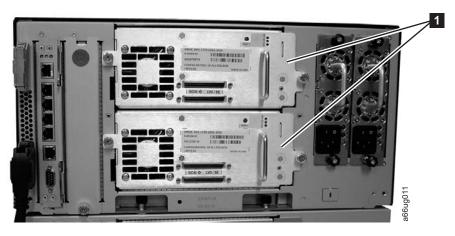
Figure 2-5. SCSI Ultrium 3 Tape Drives in the library control module
