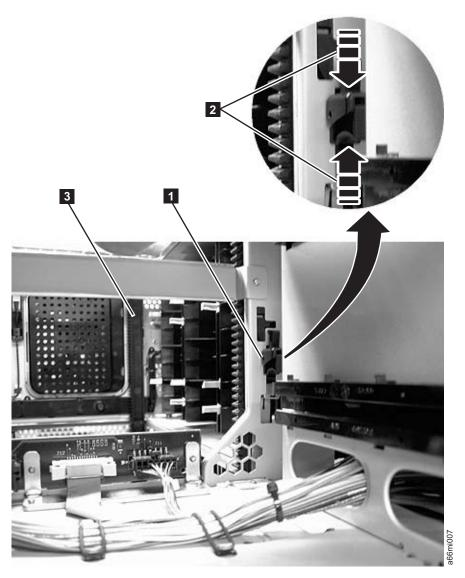
Figure 8-2. Gear racks and gear rack locking mechanism
