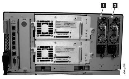
Figure 8-31. Power supplies in a control module
