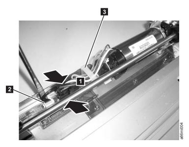
Figure 8-48. Y motor connector
