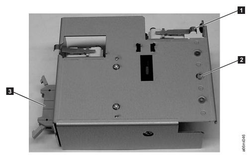
Figure 3-5. I/O Station Lock Assembly (top view)
