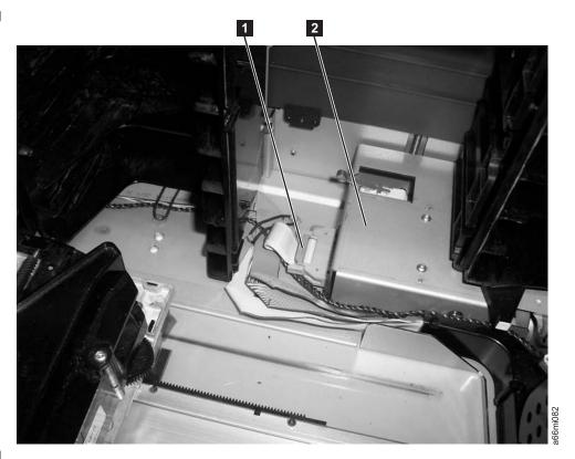
Figure 7-10. I/O Station lock assembly connector (top cover removed)
