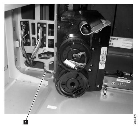
Figure 8-46. Cable Spool cable routing through enclosure wall
