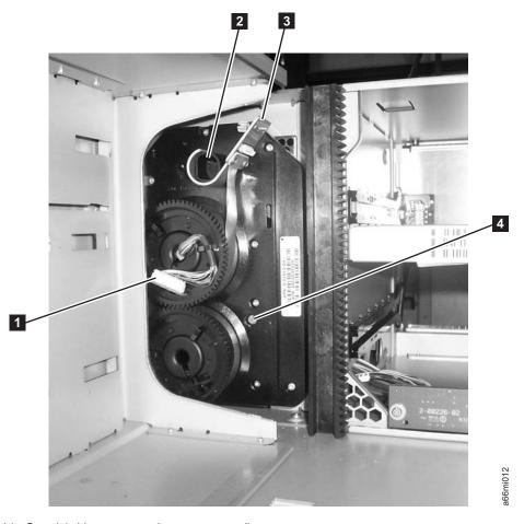
Figure 8-34. Cable Spool (with storage columns removed)
