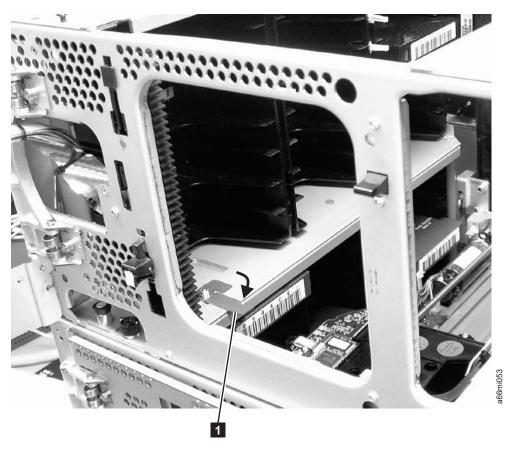
Figure 8-1. Picker locking mechanism
