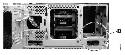
Figure 3-4. I/O Station Lock Assembly installed in the library
