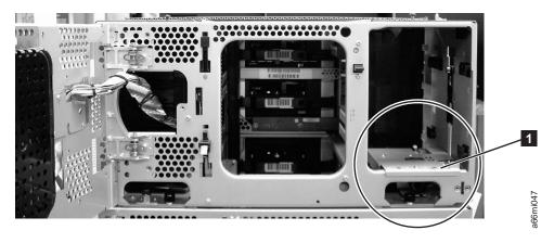
Figure 8-21. I/O Station Lock Assembly installed in library
