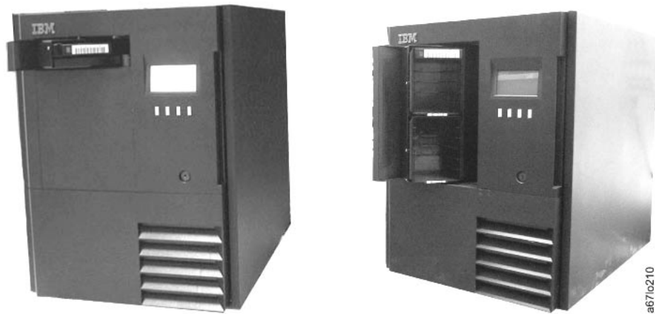
Figure 5. Types of I/O stations in the Ultrium Scalable Tape Library. The single-slot I/O station is on the left; the 12-slot I/O station is on the right.
