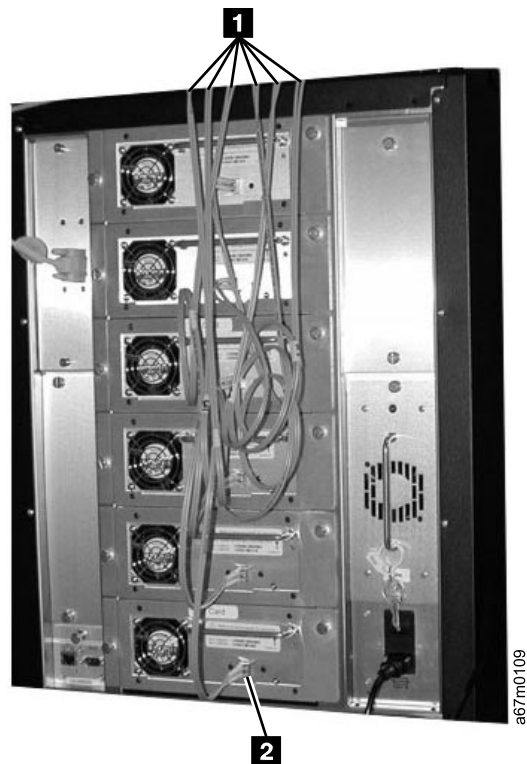
Figure 39. Making the host-to-drive connections with native Fibre Channel
