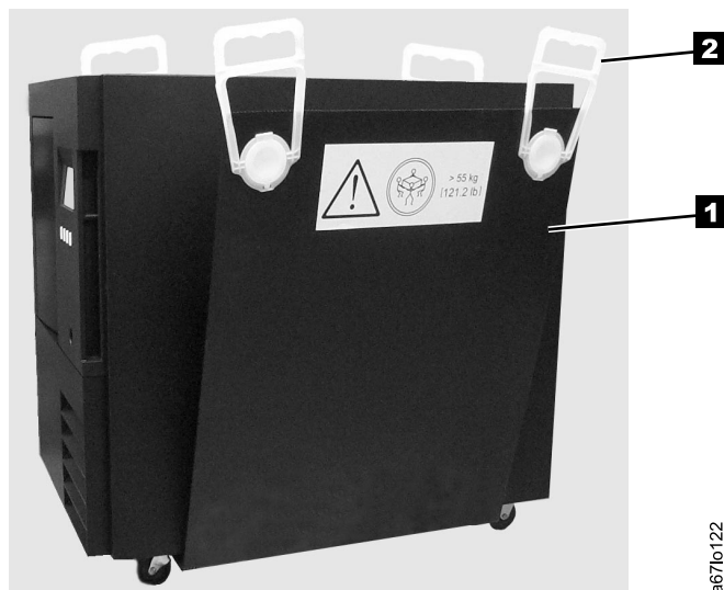
Figure 12. The sling for lifting the Ultrium Scalable Tape Library
