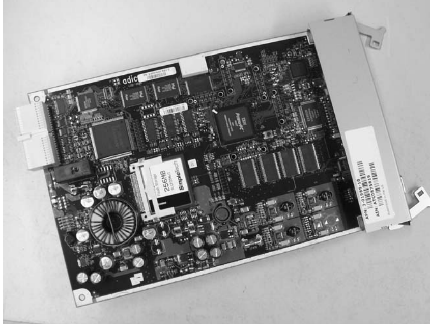
Figure 8-38. Library Control Blade (LCB)
