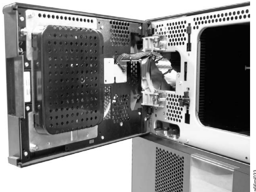
Figure 3-7. Access Door open showing back of Operator Panel
