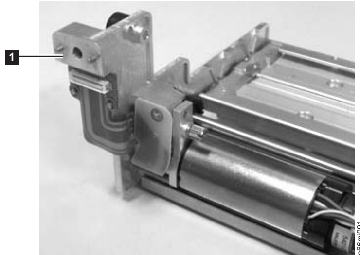
Figure 8-45. Thumbscrew securing Cable Spool
