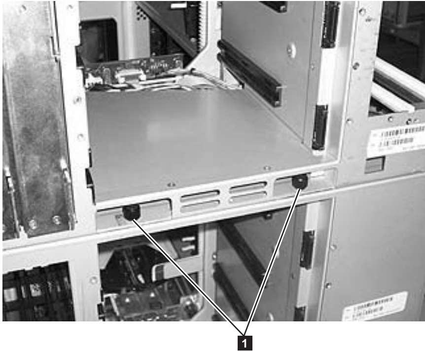
Figure 8-7. Control module rear thumb screws
