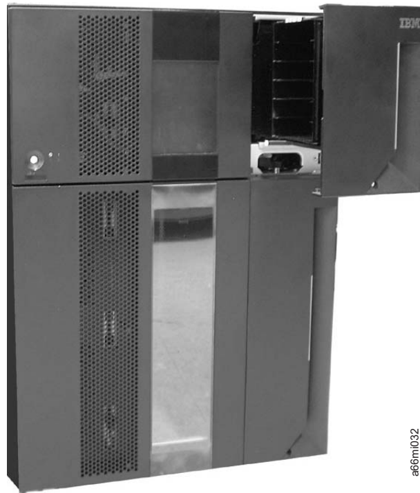
Figure 3-1. Front view of a 14U library with the I/O Station door open
