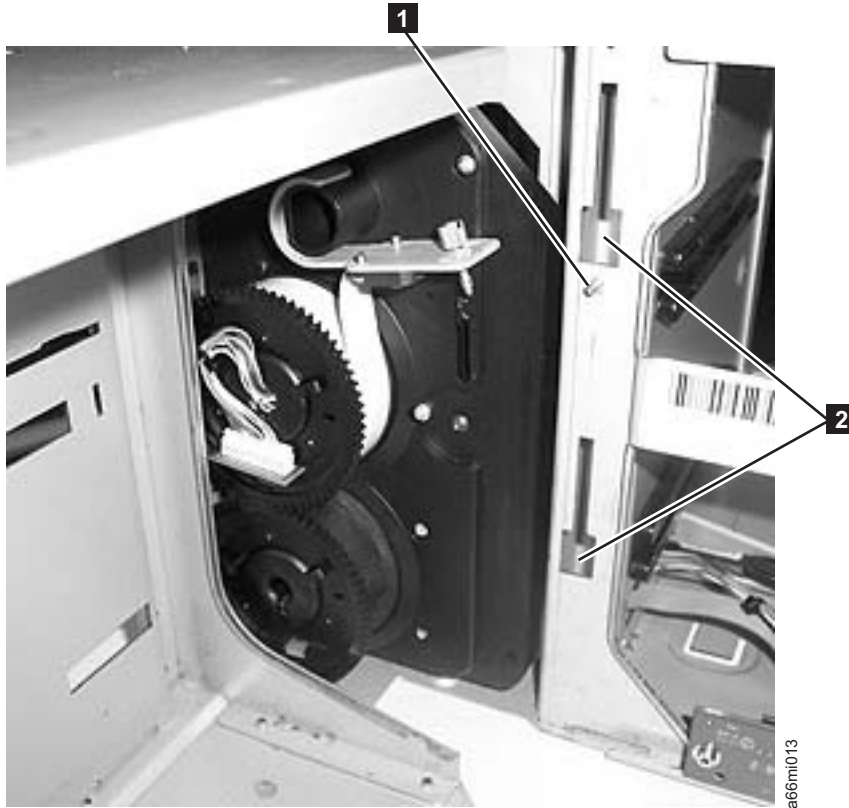
Figure 8-70. Rear gear rack location on chassis
