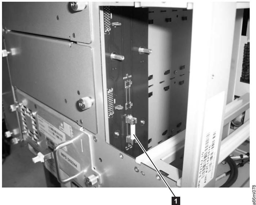
Figure 8-80. Drive power overload fuse
