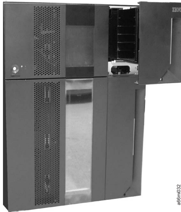
Figure 8-19. 14U library with control module I/O Station open
