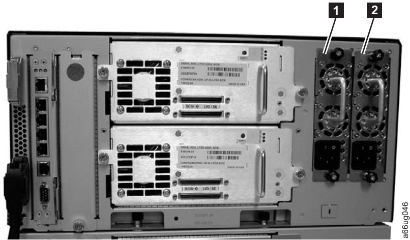
Figure 2-8. Power supply location coordinates
