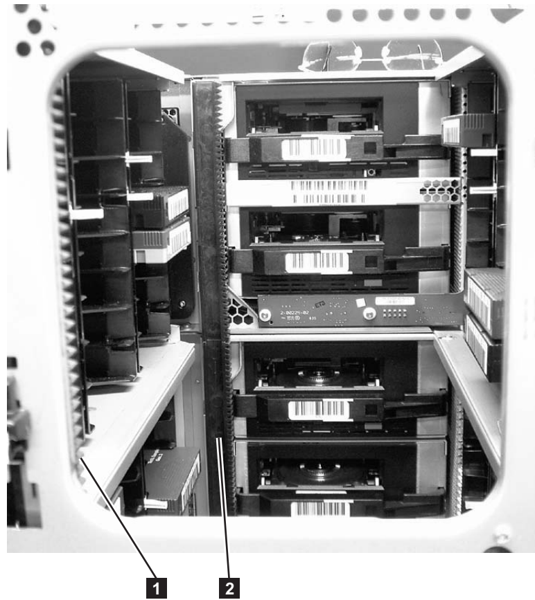
Figure 3-8. Gear racks inside the library
