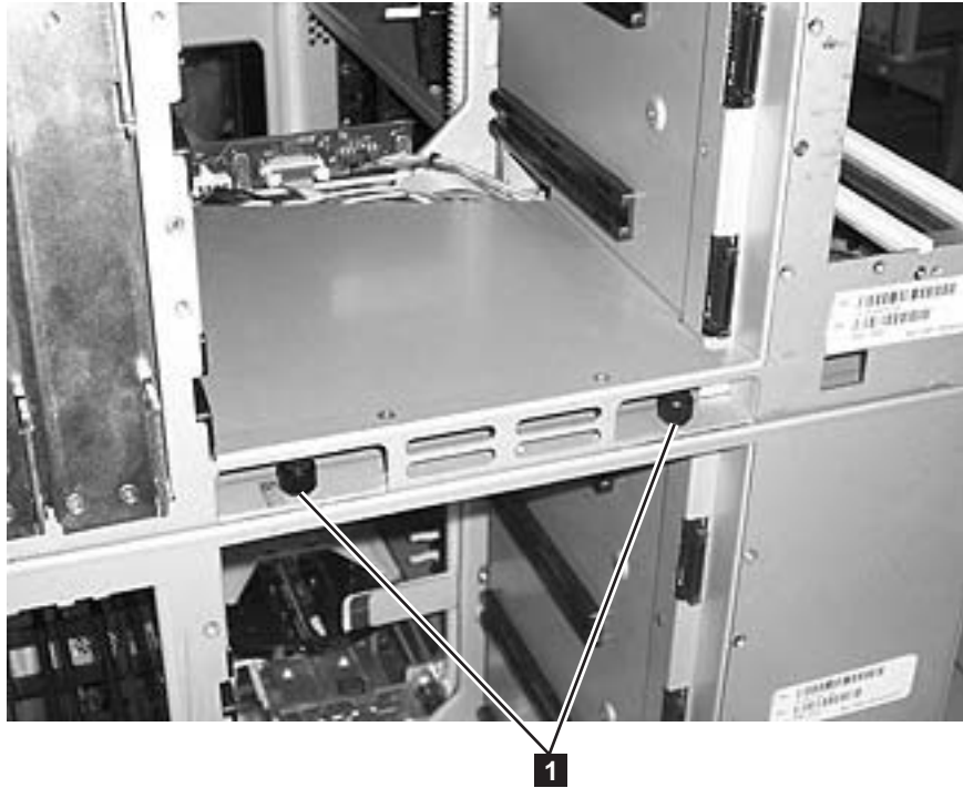
Figure 8-3. Control module rear thumb screws
