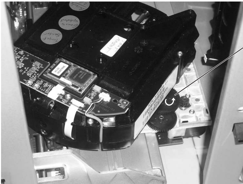
Figure 7-16. Picker rotated for drive gears access
