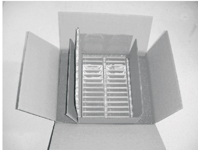
Figure 9-6. Double-boxing tape cartridges for shipping
