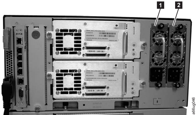
Figure 12-22. Power supplies in a control module
