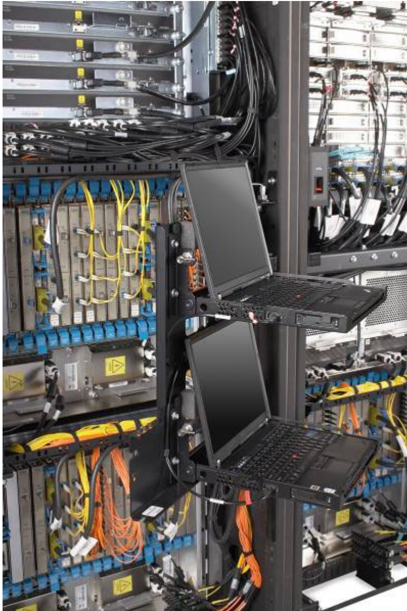
Figure 2-8 Primary and secondary Support Elements (SEs)
