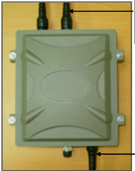
Wrap two layers of insulating tape on connectors to ensure waterproof
